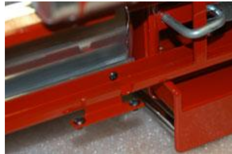
Mount the tank on the truck frame with these screws
