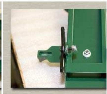
Insert the bolt into the spring and then one of the washers. Put the bolt through the hole in the frame and use another washer. Then the self tightening nut.
