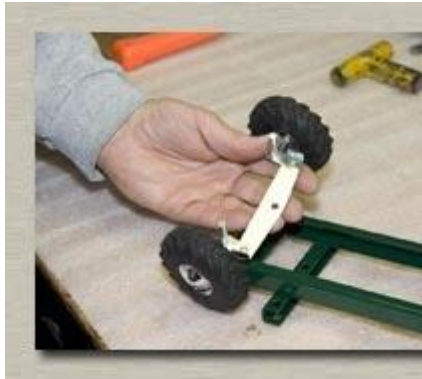
Here is the front axle and steering assembly
