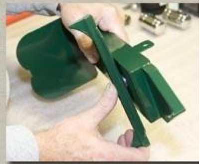
Put the bolt and bunk through the hole in the frame
