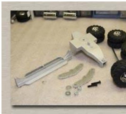
Here is the unpainted unassembled trailer with the parts needed for assembly
