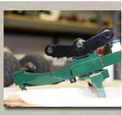
Here are the springs mounted on the trailer frame showing the position they should be.
