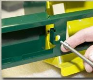
Use the 1/4" hex-head screw and slightly tighten the frame to the cab as shown.
