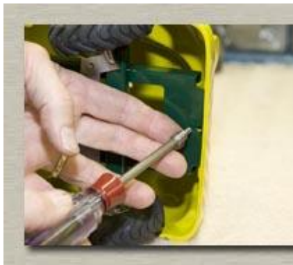
Screw the frame to the cab at the front and tighten it down.
