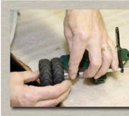
Put a sleeve on the axle and push it through the holes on the springs
