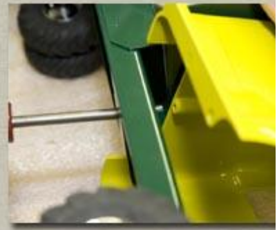
Use the 1/4" hex-head screw and slightly tighten the frame to the cab as shown.
