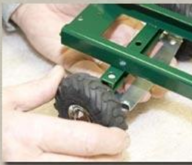
Put the spindles through the holes on the frame and make sure they turn freely
