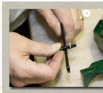
Insert the bolt into the spring and then one of the washers. Put the bolt through the hole in the frame and use another washer. Then the self tightening nut.
