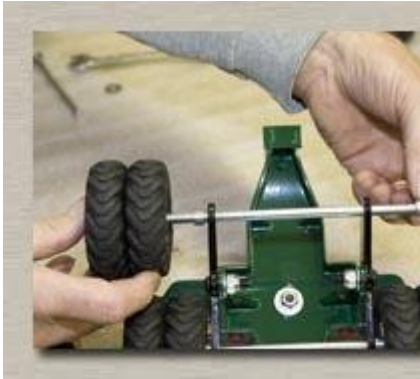
Put a sleeve on the axle and push it through the holes on the springs
