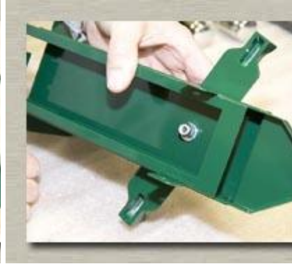
Use the self-tightening nut on the bolt
