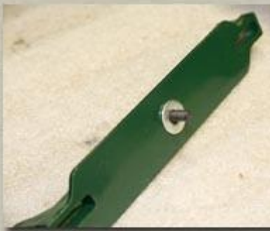
Put a washer between the log bunk and the frame
