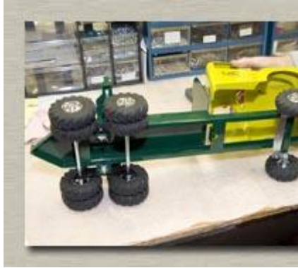
Lay the completed frame on its side and position the cab as shown
