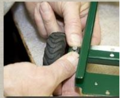
Push the two retaining clips on to the spindles to secure the axle to the frame
