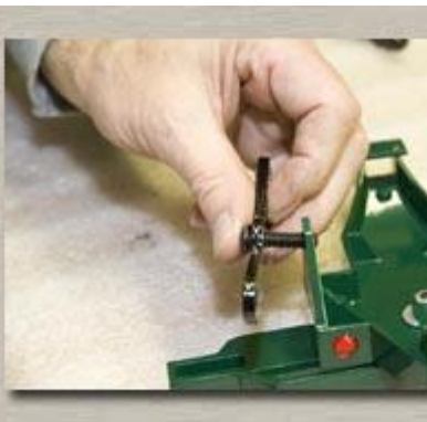
Once the trailer has been painted, you are ready to assemble the springs to the trailer frame. Note here there are no washers between the spring and the frame.
