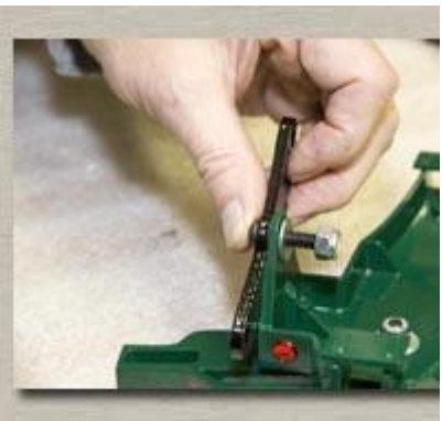
Put a washer on the inside of the trailer frame and then a self tightening nut.
