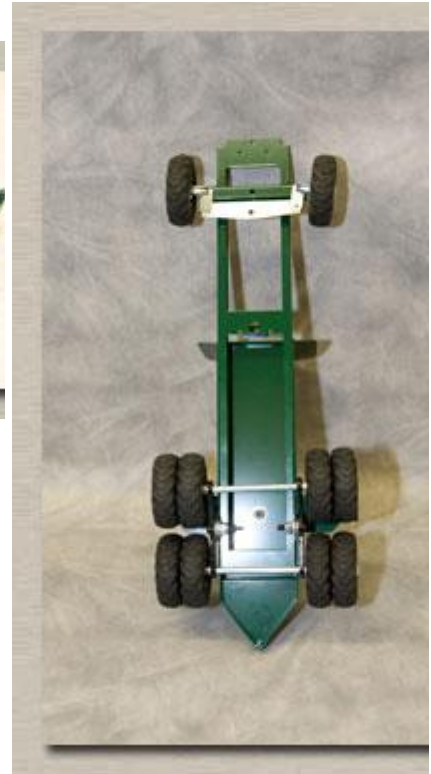
The TIMBER TOTER II frame is 1" longer than the original Timber Toter.
