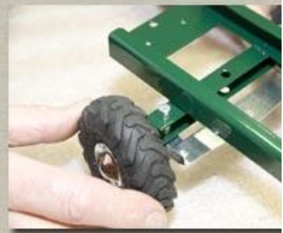
Put the spindles through the holes on the frame and make sure they turn freely
