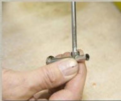
Test fit the air horn on to the "J" hook for air horn steering. Make sure that it tightens so the the horn faces the same direction as the "J" on the hook.
