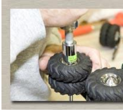
Push the hub caps on to the axles with a 5/8" socket
