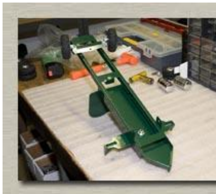
Here is the log bunk mounted on the frame ready to mount the rear springs and wheels.
