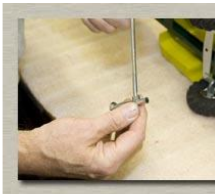
Test fit the air horn on to the "J" hook for air horn steering. Make sure that it tightens so the the horn faces the same direction as the "J" on the hook.
