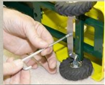
Insert the "J" hook into the hole in the steering assembly and through the hole on the hood.
