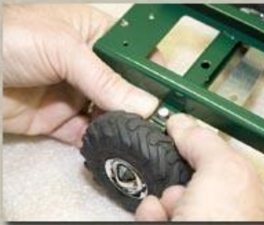
Push the two retaining clips on to the spindles to secure the axle to the frame
