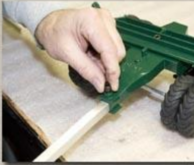
Loosen the set screw on the trailer and insert the trailer reach into the opening.
