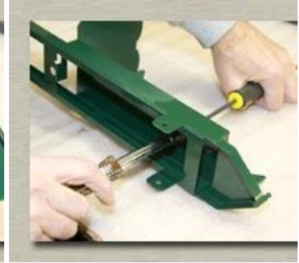
Use a 3/16" hex-head screw driver and a 7/16" socket to tighten the bunk down to the frame. Make sure that the bunk still moves freely.
