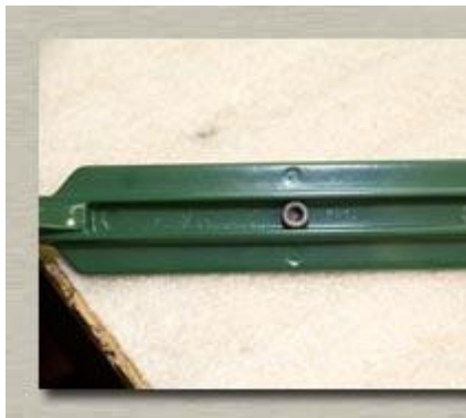
Insert the hex-head bolt into the log bunk
