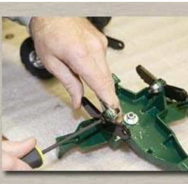
Make sure you have enough "play" in the springs so the axles can "walk."
